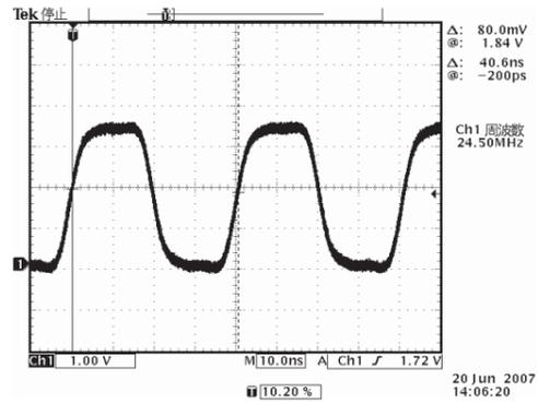
Waveform 1: Clock Waveform (24.576MHz)
