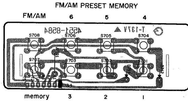
PCB-15 Tuning Switch P. C. Board
