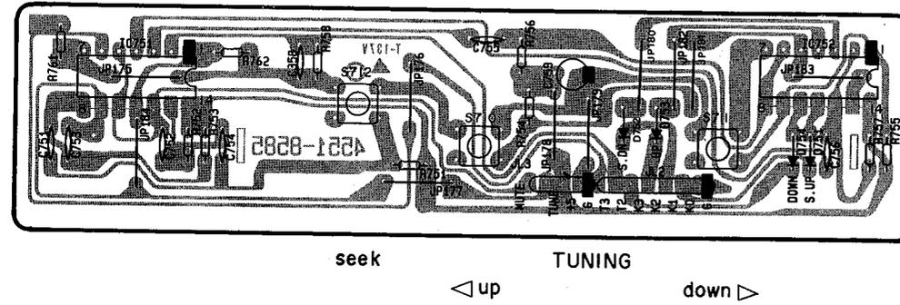
PCB-16 Antenna Terminal P. C. Board
