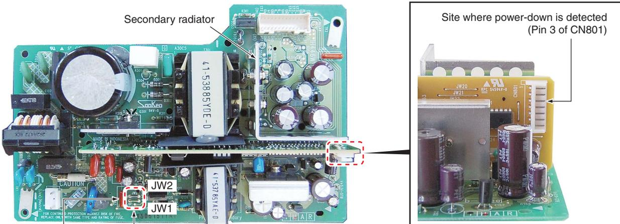
To forcibly reset latchup of STBY3.4 V, short-circuit between JW1 and JW2 (near C603), using a flathead screwdriver or similar object. If the causes of the malfunction are removed, after opening the jumpers, the unit starts up.
