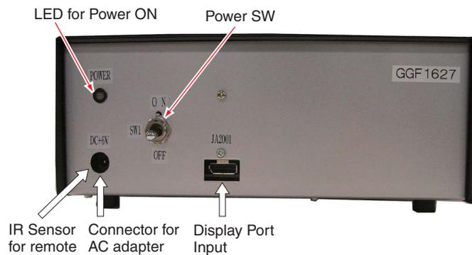
Fig.1 DP - HDMI Conversion tool (Front side)
