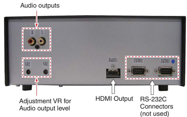
Fig.2 DP - HDMI Conversion tool (Rear side)
