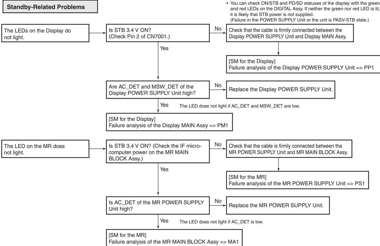
• You can check ON/STB and PD/SD statuses of the display with the green and red LEDs on the DIGITAL Assy. If neither the green nor red LED is lit, it is likely that STB power is not supplied. (Failure in the POWER SUPPLY Unit or the unit is PASV-STB state.)
