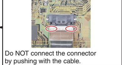
Do NOT connect the connector by pushing with the cable.
