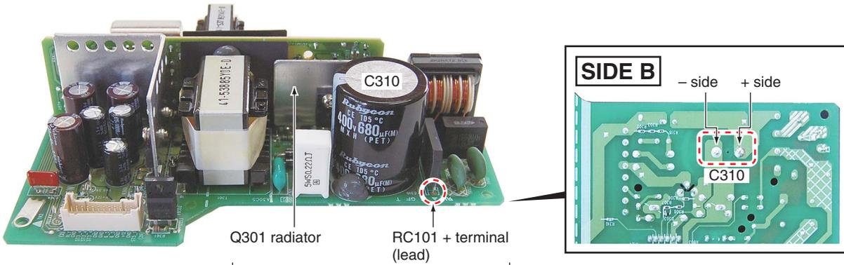
After checking that the voltage at the measurement points (equivalent to the voltage between two electrodes of C310) is under 20 V, remove the POWER SUPPLY Unit. Then, completely discharge residual charge, using resistors.
