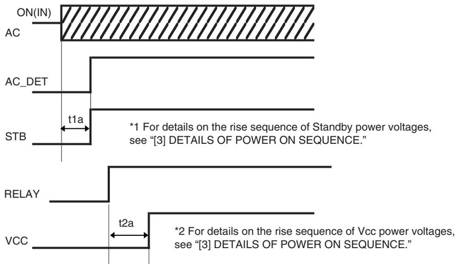
(a) Relay signal: When the POWER key on the remote control unit is pressed after that on the unit is set to ON
